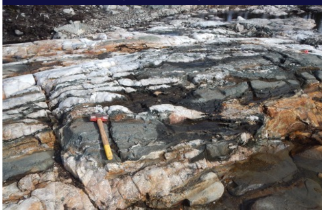
Main trench at Moby-Dick (7.78 g/t Au over 6.15 m)
